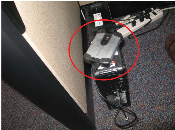
Figure 9: Unsecured Backup Media
